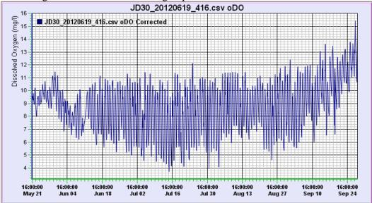
o 2012 continuous dissolved oxygen data from JD21 was compiled and corrected for fouling and calibration drift using Aquarius software.
